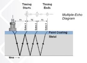
**Echo-Echo (Twin Crystal Probes)** measures through coatings of up to 1mm (0.04") thick, ideal for measuring painted metals with back wall corrosion.
