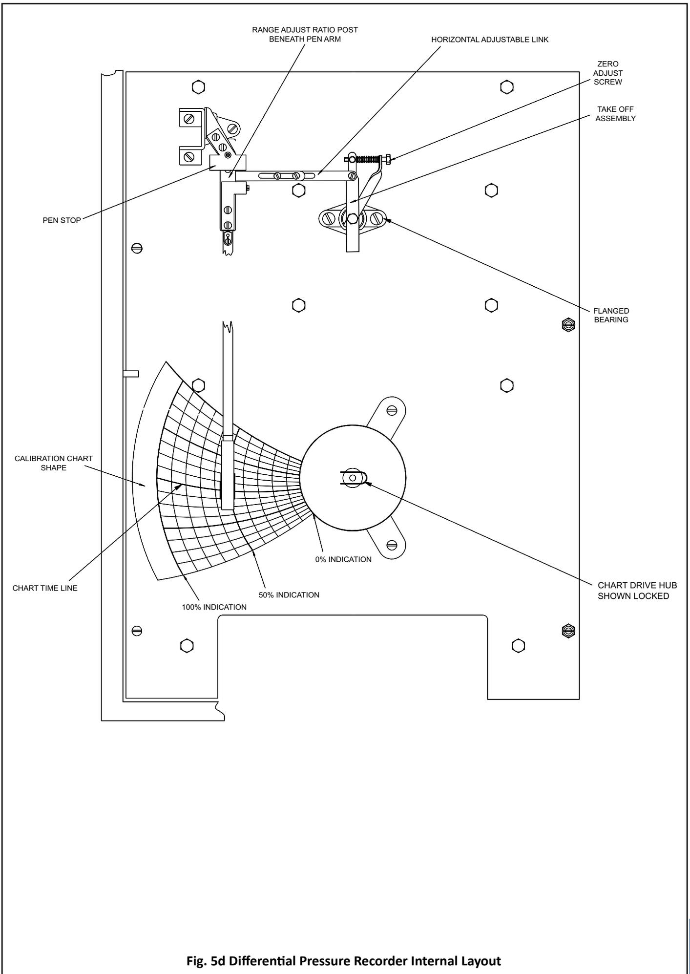
Fig. 5d Differential Pressure Recorder Internal Layout
