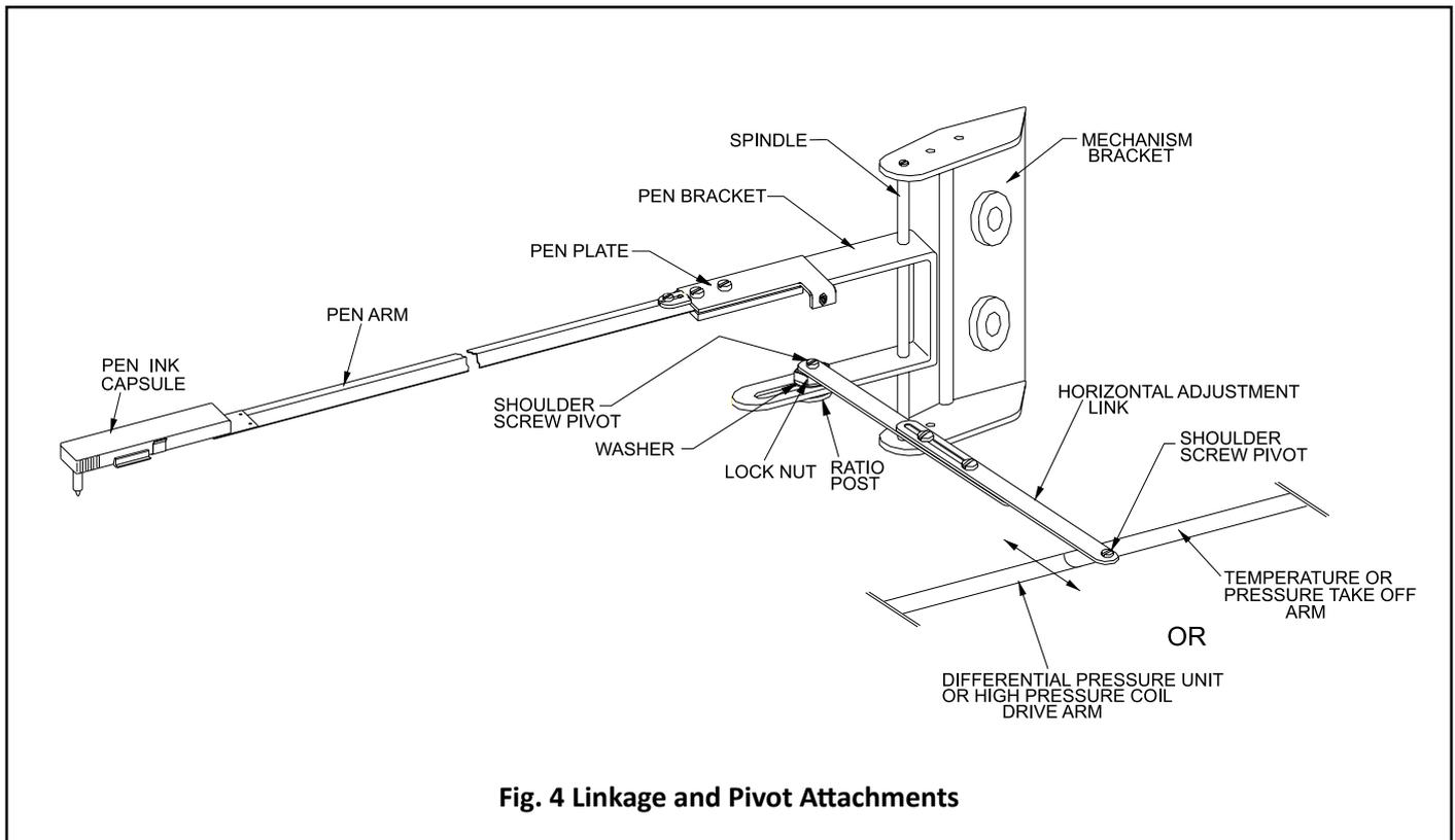
The recording pen mechanism assembly, mounted to the base plate via a bracket, provides attachment to the measuring elements.
