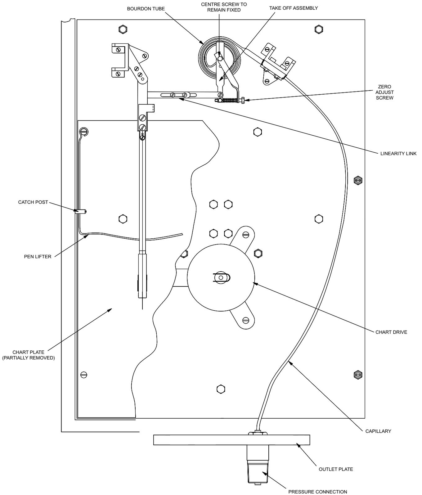
Fig. 5b Pressure Recorder Internal Layout (ranges up to 40 bar)
