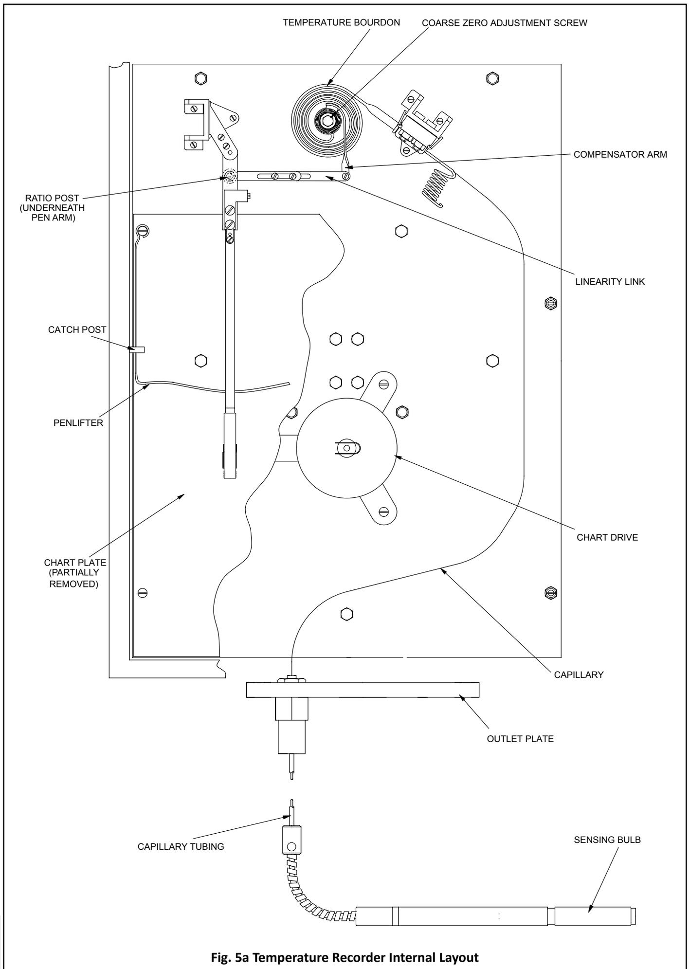
Fig. 5a Temperature Recorder Internal Layout
