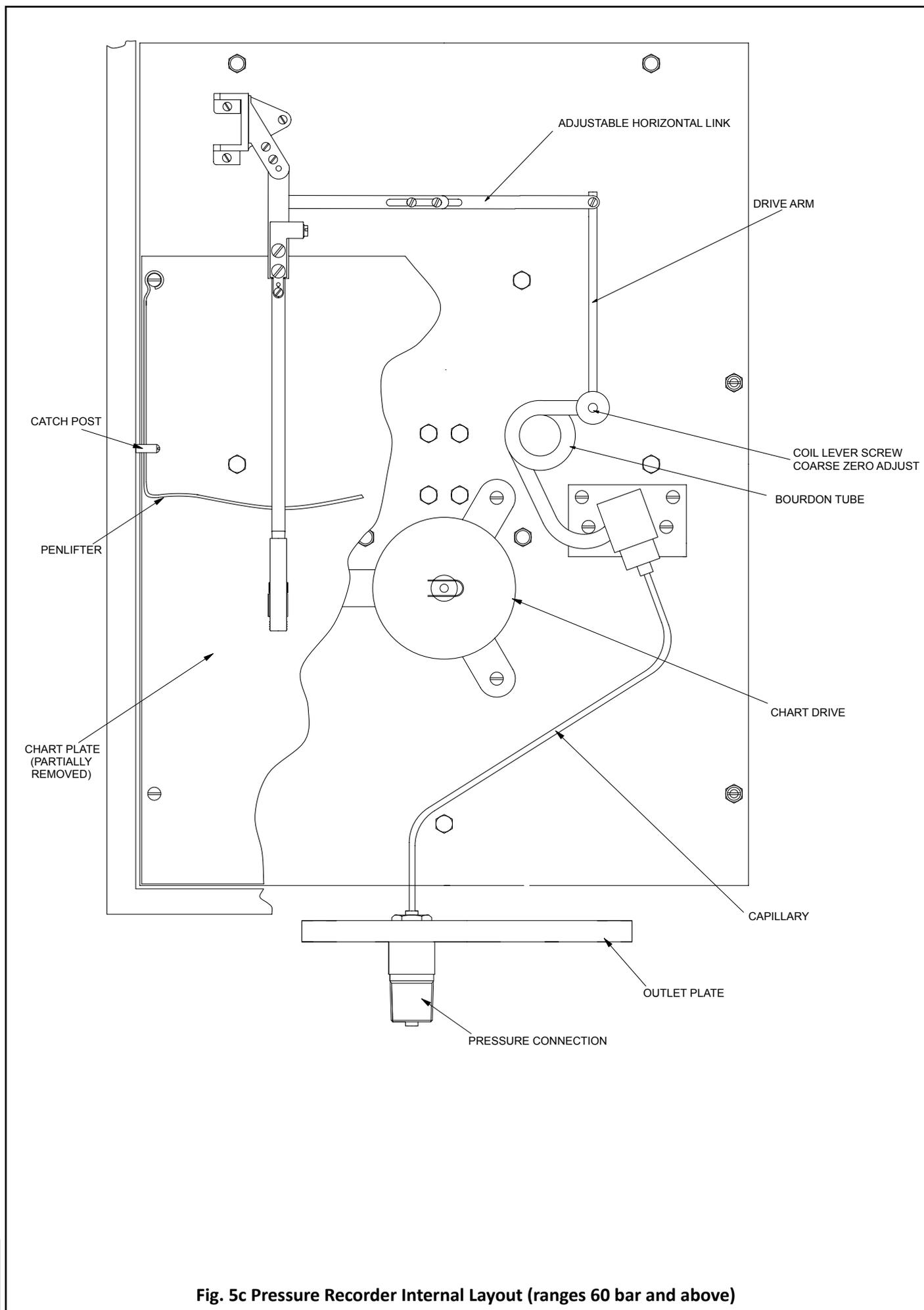
Fig. 5c Pressure Recorder Internal Layout (ranges 60 bar and above)
